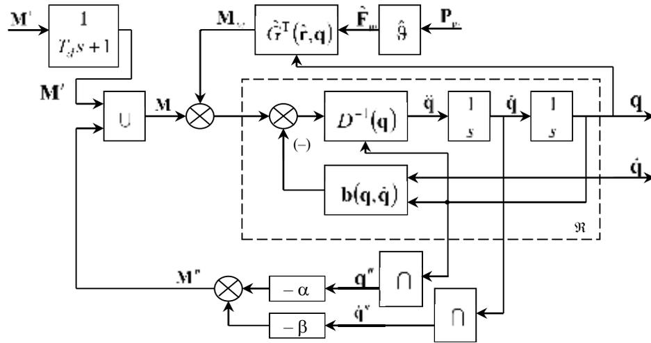
Fig. 2. Crane model structure diagram.
